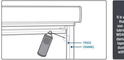
It is very important that you do not use any oil based lubricants such as WD40, as they will damage the spline tape and clog the dust that may be within the track.
