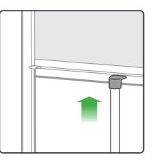
When operating the blind using a pull stick, the pull stick should only be placed in the centre of the bottom bar to push/pull the blind up or down. Pressure should only be applied on the lip of the bottom bar.
